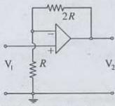
An ideal operational amplifier is connected as shown in figure. What is the output voltage  $V_2$ ?
