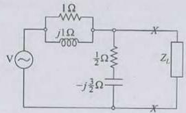
The circuit as shown in figure is connected to a load  $Z_L$  across X-X. For a maximum power transfer to the load,  $Z_L$  should be
