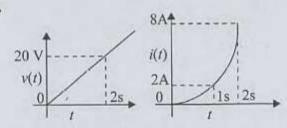
The voltage and current characteristic of an element is as shown in figure. The nature and value of the element are
