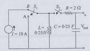
For the circuit as shown, consider that switch  $S_1$  has been in position B for a very long time and switch  $S_2$  has been open all the time. At time t=0, the switch  $S_1$  moves to position A and switch  $S_2$  closes instantaneously. What is the value of  $V_{\text{out}}$  at  $t=0^+$ , assuming initial charge on C=0?
