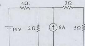
For the network shown in the figure, the current flowing through the  $5\Omega$  resistance will be
