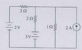
The current in the  $1\Omega$  resistor in the network as shown is
