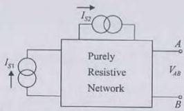
In the network as shown, with  $I_{S1} = 5$ A,  $I_{S2} = 10$ A,  $V_{AB} = 120$ V, and with  $I_{S1} = 10$ A,  $I_{S2} = 5$ A,  $V_{AB} = 15$ V. What is the value of k to describe  $I_{S1} = k I_{S2}$ , such that  $V_{AB} = 0$ ?
