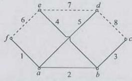
A network graph with its tree shown by firm lines is given in the figure. The fundamental cut-set for the tree-branch number 2 is
