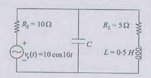
For the circuit as shown, what is the value of C that leads to maximum power transfer to the load, if the value of L is  $0.5 \,\mathrm{H}$ ?
