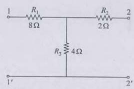
The Z parameters  $Z_{11}$ ,  $Z_{12}$ ,  $Z_{21}$  and  $Z_{22}$  for the circuit as shown in figure, respectively, are
