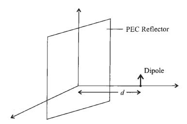
Derive an expression for the half-power beamwidth of the x-y plane pattern of a  $\frac{\lambda}{2}$  dipole placed in front of a flat reflector as shown. What is the half-power beamwidth if  $d = \frac{\lambda}{4}$ ?
