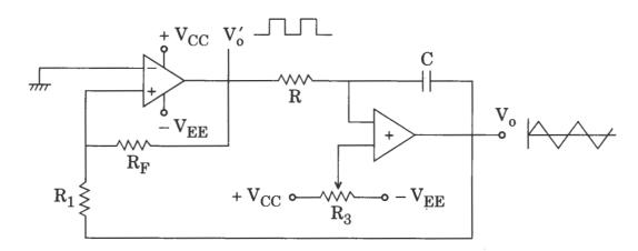
(ii) Design a square wave generator as shown in the figure below, so that duty cycle is 50% and  $f_o$  = 2.5 kHz. Assume  $V_{CC}$  = 12 V and C = 0.1  $\mu F$ .
