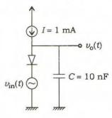
Representing the diode by its small signal resistance  $r_d$ , which is a function of I, sketch the circuit for determining  $v_o(t)$  and thus find out cutoff frequency  $f_H$ . (Assume  $V_T=25\,\mathrm{mV}$  at room temperature)
