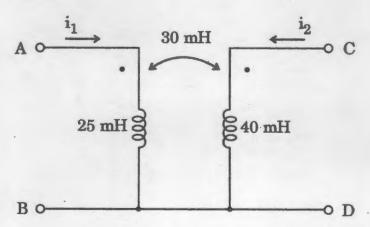
Establish the equivalence between the network and its T equivalent.
