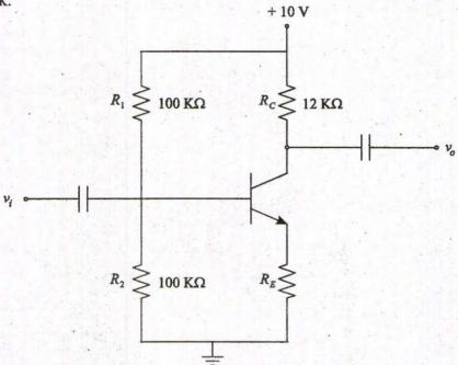
(i) Common emitter (CE) amplifier shown in the figure has voltage gain 400 when  $R_E = 0$ . Stability is brought through negative feedback by adding resistor  $R_E$ . Find the value of resistor  $R_E$  using feedback concepts so that final voltage gain is equal to 200.
