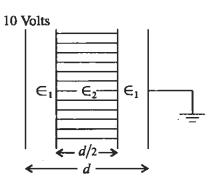
A parallel plate capacitor consisting of two dielectric materials is shown in figure. The middle dielectric slab is placed symmetrically with respect to the plates. If the potential difference between one of the plates and nearest surface of dielectric interface is 4 volts, determine  $\frac{\epsilon_1}{\epsilon_2}$ . Assume parallel plate capacitor has an electrode area of A m<sup>2</sup>.
