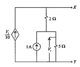
Determine the value of Load Resistance  $R_L$  to be connected across terminals X-Y to receive maximum power. Also, obtain the value of this maximum power.
