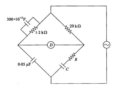
For the bridge circuit shown determine the values of R and C. Derive the formula used.
