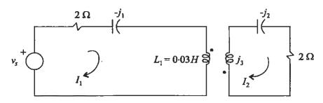
For the network shown,  $v_s = 24\sqrt{2}\sin 100t$ , coefficient of coupling  $k = \frac{1}{3}$  between two coupled coils.
