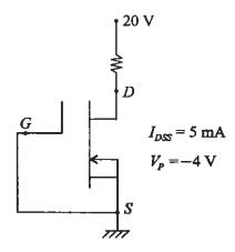
Write the equation related to the drain current  $(I_D)$  and Gate to source voltage  $V_{GS}$  explaining all the parameters for
