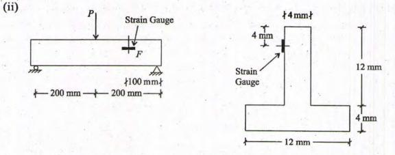
A small T-section is used in inverted position as a beam and is shown in figure over a span of 400 mm. If due to the application of forces shown, the longitudinal strain gauge at F registers a compressive strain of 1500 microstrains, determine the magnitude of P. Take E = 200 GPa. 10
