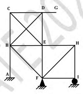
If the axial deformations are neglected, the degree of kinematic indeterminacy is \_\_\_\_\_ (in integer).
