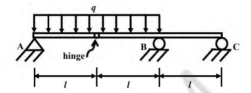
Considering the upward reactions as positive, the support reactions are
