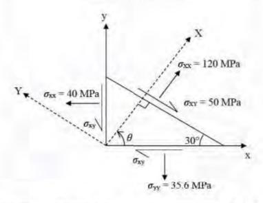
The absolute magnitude of the shear stress component \(\sigma\_{\*v}\) (in MPa, round off to one decimal place) in x-y coordinate system is \_
