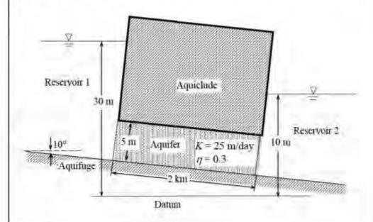
If water in Reservoir 1 is contaminated then the time (in days, round off to one decimal place) taken by the contaminated water to reach to Reservoir 2 will be
