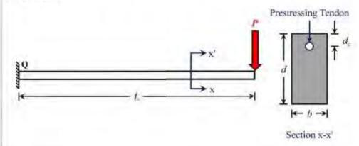
If the concentrated load, P = 5 kN, the resultant stress (in MPa, in integer) experienced at point 'Q' will be \_\_\_\_\_
