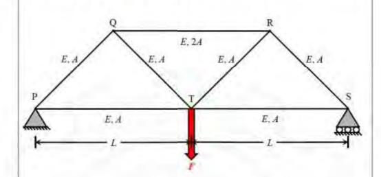
If load,  $F = 10\sqrt{3}$  kN, moment of inertia,  $I = 8.33 \times 10^6$  mm<sup>4</sup>, area of cross-section,  $A = 10^4$  mm<sup>2</sup>, and length, L = 2 m for all the members of the truss, the compressive stress (in kN/m<sup>2</sup>, in integer) carried by the member Q-R is \_\_\_\_\_
