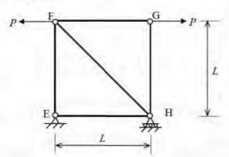
If  $R = 500 \times 10^3$  kN, P = 150 kN and L = 3 m, the magnitude of the horizontal displacement of joint G (in mm, round off to one decimal place) is
