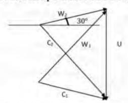
The blade speed (U) at the mean radius of the rotor is \_\_\_\_\_\_m/s (round off to two decimal places).
