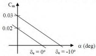
Based on the result presented in the figure above, the value of elevator control power  $(C_{m\delta e})$  in per radian will be \_\_\_\_\_ (in three decimal place).
