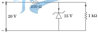
Give reason to explain why n and p regions of a Zener diode are heavily doped. Find the current through the Zener diode in the circuit given below: (Zener breakdown voltage is 15 V)
