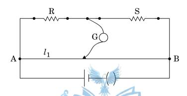
An unknown resistance X is now connected in parallel to the resistance S and the balance point is found at a distance  $l_2$ . Obtain a formula for X in terms of  $l_1$ ,  $l_2$  and S.
