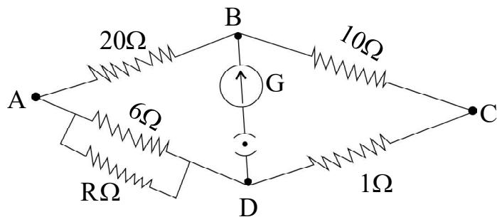
Calculate the value of unknown resistance  $R$  in given circuit. If wheatstone bridge is in balanced condition.
