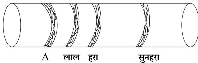
In given diagram value of carbon resistor is  $22 \times 10^5 \Omega \pm 5\%$ . Write colour of first ring A.
