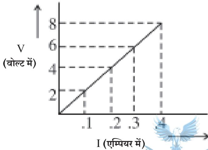
Determine the resistance of a resistor with the help of given V-I graph. [1]
