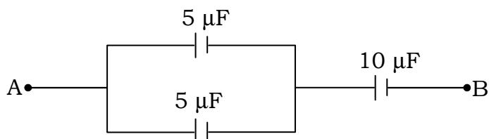
What is capacitance of a capacitor ? Calculate equivalent capacitance between points A and B :
