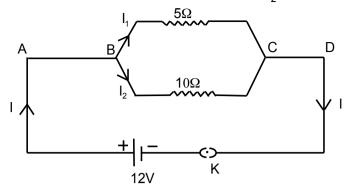
In the given circuit diagram calculate the current  $l_2$  through the resistor of  $10\Omega$ .
