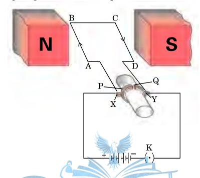
As shown in the figure, the current in the coil ABCD flows from A to B in the arm AB and C to D in the arm CD.
